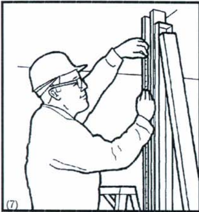
(7) Scribe line on structural column at height "Y" as measured in step (6).
