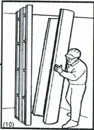
(10) Locate column cover half as identified by the larger, indented vertical flange and position over scribed circular line on floor.
