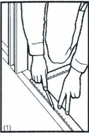
(1) Locate center of structural column and scribe a line on both sides which extend further than the base to be installed later.
